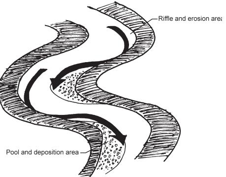
creating new stream banks and habitat, while erosion occurred in the riffles where water movement was faster, ca ing wider curves in the river and carr ing sediment downstream.
