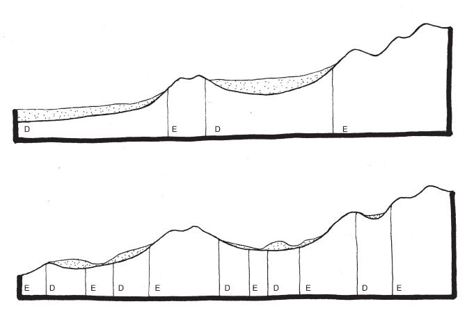
E- Erosion D- Deposition
